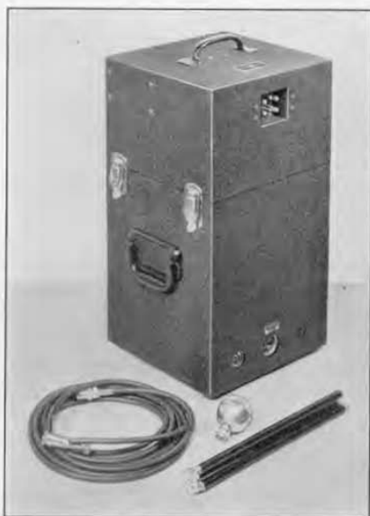
FIGURE 2. Lamp housing and power supply lock together in a convenient assembly for transportation.
