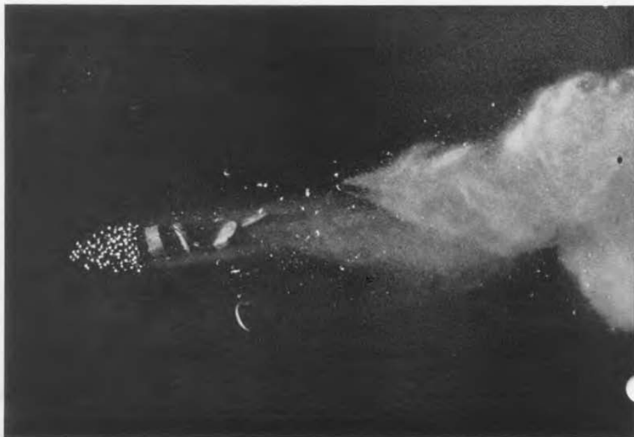
FIGURE 3. Microflash photo of the explosion of a shotgun shell as it leaves the muzzle of gun, which is out of the picture at the right. Note that the wads can be seen as well as the cluster of shot.
