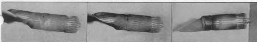
FIGURE 4. Photographs of three rounds of ammunition showing both yaw and erratic behavior of windshields.
